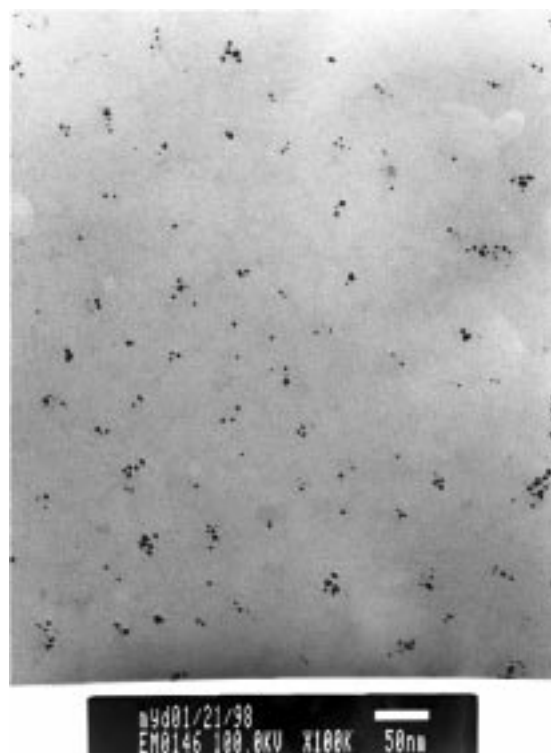
Figure 2. TEM of the polymer-grafted palladium cluster deposited on a 200 mesh copper grid covered with colosion.
